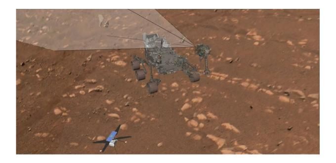
This computer simulation shows NASA's Perseverance Mars rover taking its first selfie, on April 6, 2021. The point of view of the rover's WATSON camera is included to show how each of the 62 images were taken before being sent to Earth and stitched together into the selfie. Credit: NASA/JPL-Caltech
