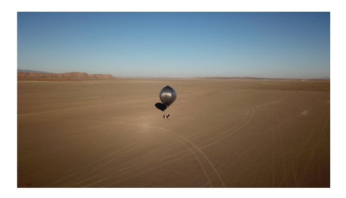
Four "heliotrope" balloons were flown near Ridgecrest, California, after a series of earthquakes rattled the region in July, 2019. By attaching barometers to the balloons, researchers from JPL and Caltech hoped to detect the sound of one of the aftershocks. Credit: NASA/JPL-Caltech
