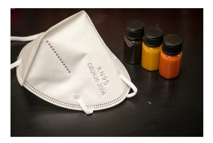
The N95 prototype mask made with dielectric fabric, with bottles of copper nanoparticles of various colours in the background. Credit: Nanyang Technological University
