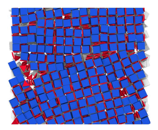
Computer simulations identified the conditions under which nanoscale cubes would self-assemble into a grid, incorporating flat triangular shapes between them. This technique could help enable new kinds of materials with new properties. Credit: Glotzer Lab, University of Michigan
