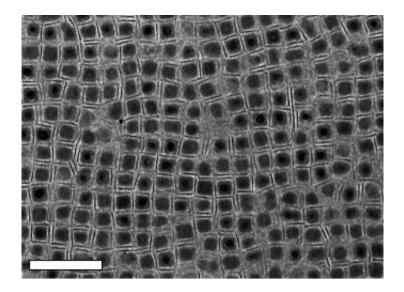
Cubes of lead telluride and triangles of lanthanum fluoride self-assembled into a grid in the lab, when the researchers followed the conditions discovered through the computer simulations. This technique could help enable new kinds of materials with new properties. The scale bar on the electron microscope image is 100 nanometers. Credit: Murray Lab, University of Pennsylvania
