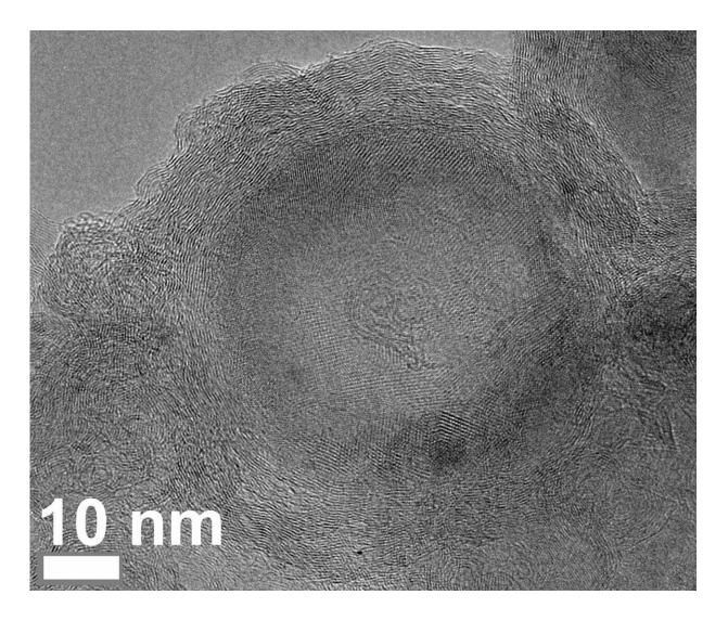
An electron microscope image shows a late stage in the evolution of carbon and fluorine atoms under flash Joule heating. The carbon atoms form concentric shells around a nanodiamond core. As heating proceeds, the diamond phase is replaced by the shell. Credit: Tour Group/Rice University
