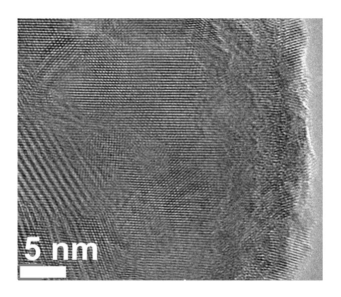
A transmission electron microscope image shows a nanodiamond lattice. Rice University chemists used their flash Joule heating technique to control the phase evolution and doping of carbon. Credit: Tour Group/Rice University
