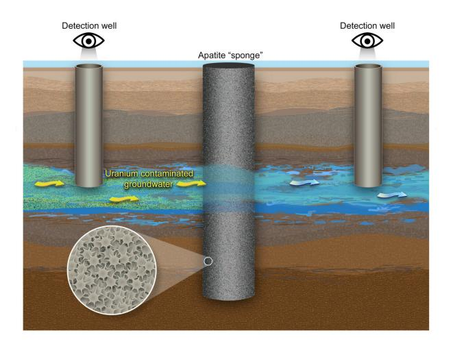
A graphical illustration of the apatite remediation test to absorb uranium conducted by Sandia, Lawrence Berkeley and Pacific Northwest national laboratories researchers. Credit: Sandia National Laboratories
