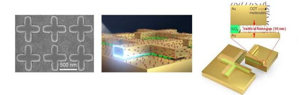
(Left) SEM image of the metamaterial absorber developed by KIMM and UNIST. Top view shows cross-shaped antenna. (Center) Side view of the microstructure of the metamaterial absorber developed by KIMM and UNIST. (Right) Structure of the metamaterial absorber developed by KIMM and UNIST. Figure shows 10 nm vertical nanogaps. Credit: The Korea Institute of Machinery and Materials (KIMM)
