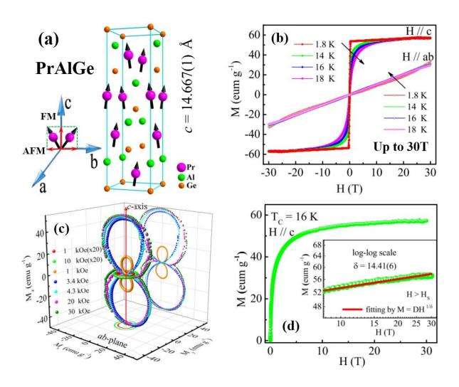
Figure 1. (a) Crystal and magnetic structures of PrAlGe; (b) M(H) curves up to high magnetic field of 30T; (c) angular-dependent magnetization; (d) critical isothermal analysis under high magnetic field. Credit: ZHANG Lei
