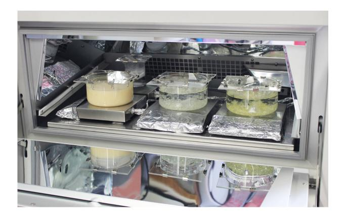
Samples of plastic particles in the weathering facility. Credit: C. Wißler
