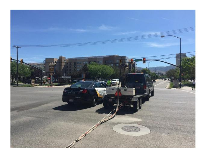
Sensors for an active seismic source experiment are contained in a firehose as the researchers drive through downtown Salt Lake City, Utah. Credit: Lee Liberty
