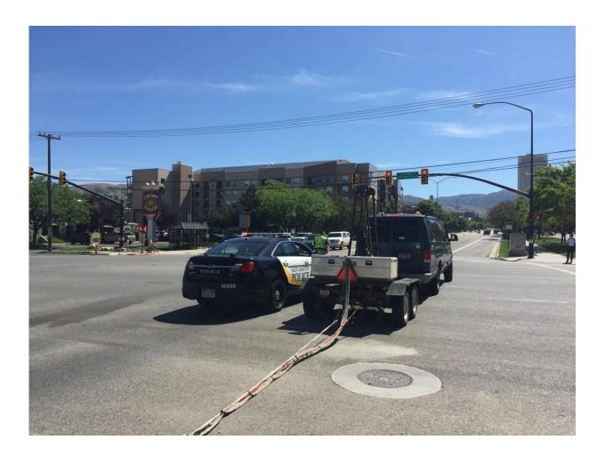
Sensors for an active seismic source experiment are contained in a firehose as the researchers drive through downtown Salt Lake City, Utah. Credit: Lee Liberty
