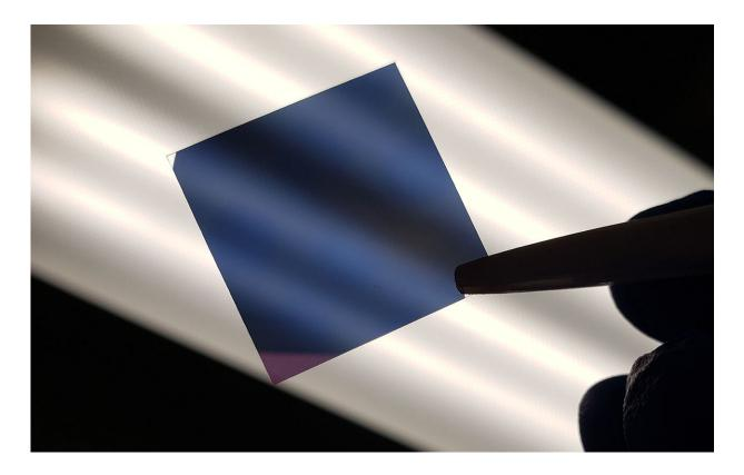
This light-shrinking material turns a conventional light microscope into a superresolution microscope. Credit: Junxiang Zhao
