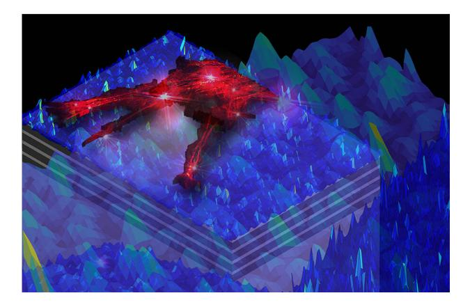
Artistic rendering of the new super resolution microscopy technology. Animal cells (red) are mounted on a slide coated with the multilayer hyperbolic metamaterial. Nanoscale structured light (blue) is generated by the metamaterial and then illuminates the animal cells. Credit: Yeon Ui Lee
