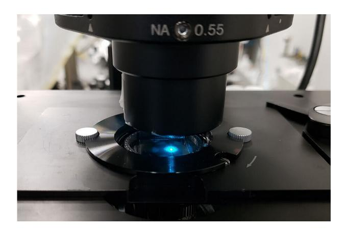
The material mounted on the stage of an inverted microscope. Credit: Junxiang Zhao
