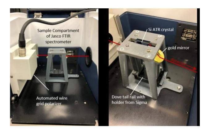
3D printable optical setup with built-in sample chamber for a FT-IR spectrometer. Sample is put on the Si ATR crystals for measurement. Credit: ©M. Takahashi & K. Okada, Osaka Prefecture University
