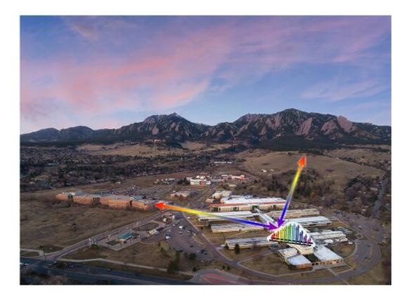
NIST researchers used a laser frequency-comb instrument (illustration at lower right) to simultaneously measure three airborne greenhouse gases -- nitrous oxide, carbon dioxide and water vapor -- plus the major air pollutants ozone and carbon monoxide over two round-trip paths (arrows) from a NIST building in Boulder, Colo., to a reflector on a balcony of another building, and another reflector on a nearby hill. Credit: N. Hanacek/NIST
