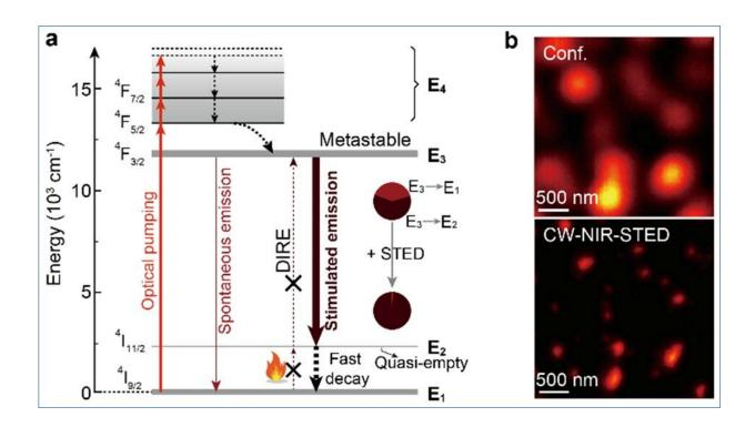
Figure (a) shows the proposed optical emission depletion mechanism of the near infra-red (NIR) downshifting luminescence in the neodymium-mediated stimulated-emission depletion (STED) process. Figure (b) compares the images obtained from conventional confocal imaging and STED imaging using the lanthanide nanoparticles, with better contrast in the latter technique. Credit: LIANG Liangliang
