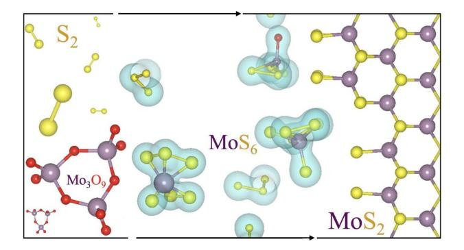
Three gas-phase molecules react at high temperatures during chemical vapor deposition to form molybdenum disulfide, a two-dimensional semiconductor that could find use in next-generation electronics. In this illustration, molybdenum atoms are purple, oxygen is red and sulfur is yellow. Credit: Jincheng Lei/Rice University
