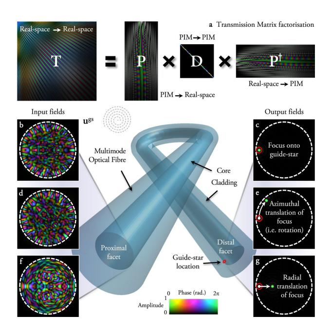
Fig. 1: Field transformations through multimode fibres. From: Memory effect
