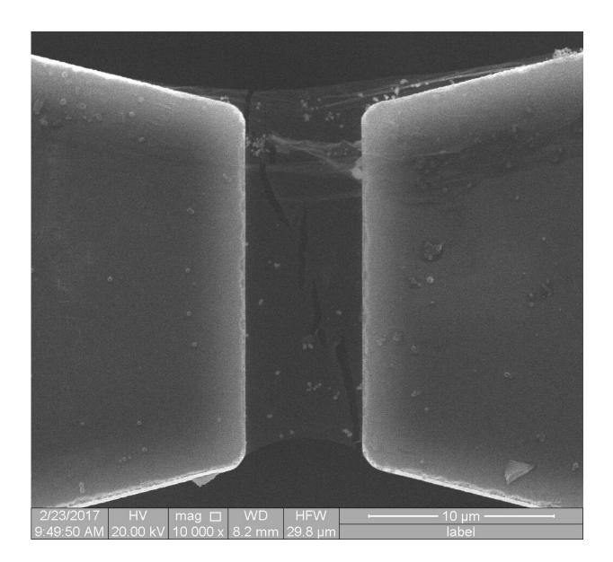
A scanning electron microscope image shows branched cracks in a single crystal of 2D hexagonal boron nitride (h-BN). Experiments and computational
