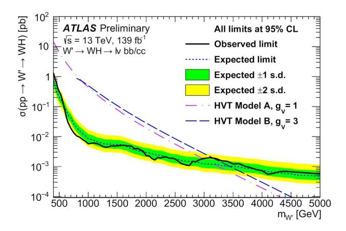
Figure 2: Combined 95% observed (expected) exclusion limits on the production cross section of the W' boson are shown by the black (blue) line. The purple and blue dashed lines indicate the theoretical cross section vs mass for a version of the HVT theory with a specific value of the coupling to the Standard Model W boson. All W' masses below and to the left of each dashed line are excluded for that value of the coupling. Credit: ATLAS Collaboration/CERN
