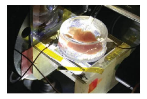
A heart removed from a chicken embryo sits in the CAGE device, which uses a sheet of graphene under the heart to measure tiny electrical fields produced when the heart beats. Credit: Halleh Balch, Allister McGuire and Jason Horng
