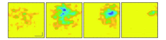
This sequence of images, each separated by 5 milliseconds, shows changes in the electric field pattern on the surface of an embryonic chicken heart during a single beat, measured by a laser bouncing off a graphene sheet lying beneath the heart. The images are about 2 millimeters on a side. Credit: UC Berkeley/Halleh Balch, Alister McGuire and Jason Horng
