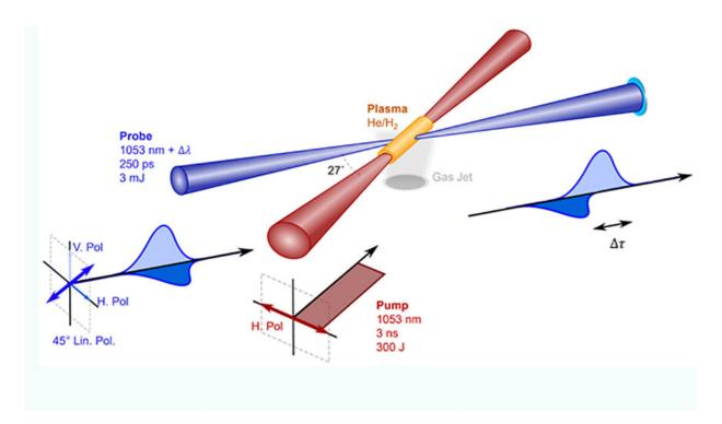
This image depicts the experiment schematic where the probe and pump beams interact in a plasma formed by the pump. Credit: Lawrence Livermore National Laboratory
