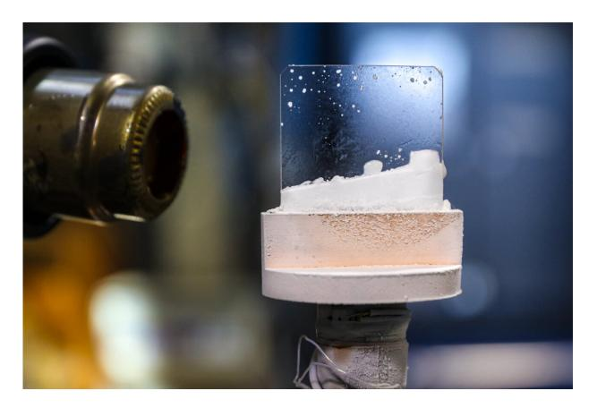
Scientists created this exotic "outer space" ice by freezing a stream of heavy water (D2O) molecules on a sapphire plate that is cooled to about -414 degrees F in a vacuum chamber. Credit: ORNL/Genevieve Martin
