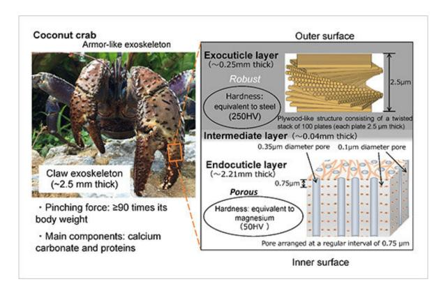
Schematic diagram showing the cross-sectional structures of the coconut crab claw exoskeleton. Credit: National Institute for Materials Science
