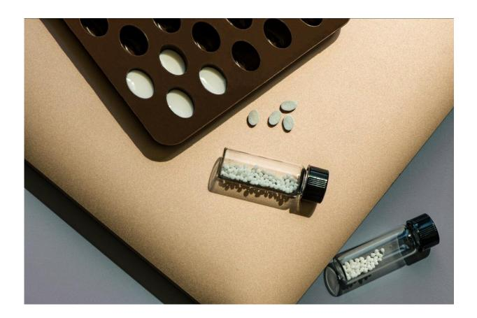
MIT chemical engineers have devised a new way to formulate hydrophobic drugs by turning them into a nanoemulsion, which can be poured into a mold and dried into tablets. The nanoemulsion can also be used to form small particles, seen in the vials. Credit: Felice Frankel
