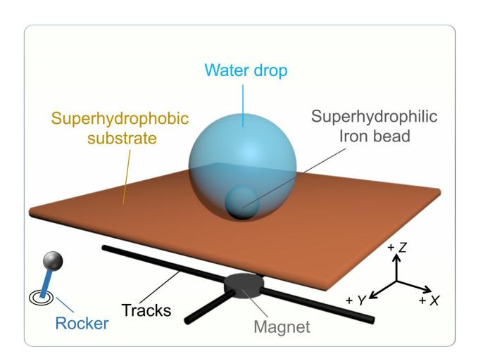
A schematic illustration of magnetically driven Hydrobot on a superhydrophobic surface. Credit: Yifan Si
