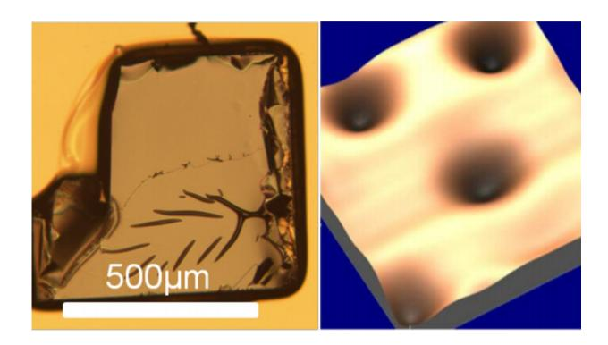
On the left: a crystal coated in gold -- the gold coating allows the magnetic imaging tool to get within nanometers of the material's surface. On the right: a magnetic picture of a segment of the crystal showing the vortices (dark holes) that were studied. Credit: University of Bath
