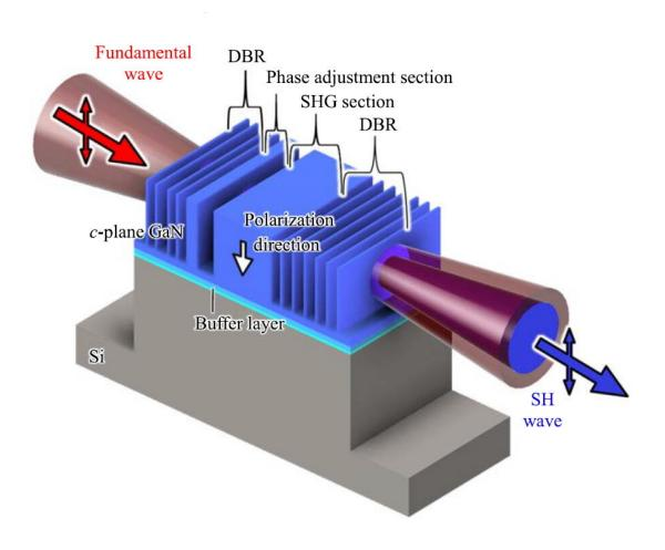
Fig. 1 Schematic of GaN monolithic microcavity Second-Harmonic Generation (SHG) device on a Si pedestal structure. Credit: Osaka University
