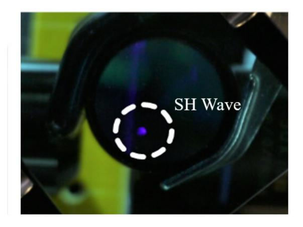
Fig. 3 Digital camera image of blue second harmonic light emission with a wavelength of 428 nm using an IR cutoff filter. Credit: Osaka University
