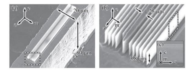
Fig. 2 SEM images of SHG device. (a) and (b) GaN monolithic microcavity SHG device on a Si pedestal structure, (c) GaN sidewall view of SHG device. Credit: Osaka University
