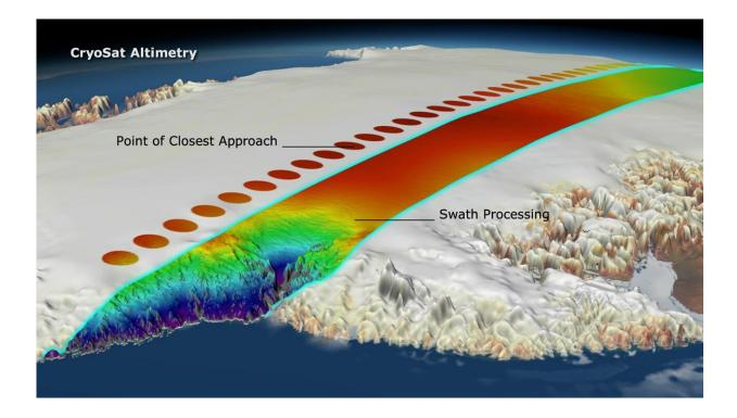
The technique of swath processing differs from conventional radar altimetry.
