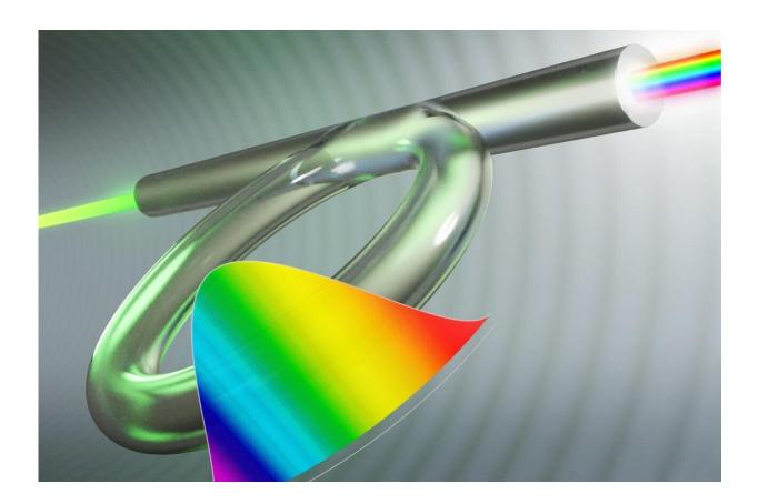
An illustration of the optical fiber Kerr resonator, which Rochester researchers used with a spectral filter to create highly chirped laser pulses. The rainbow pattern in the foreground shows how the colors of a chirped laser pulse are separated in time. Credit: University of Rochester / Michael Osadciw
