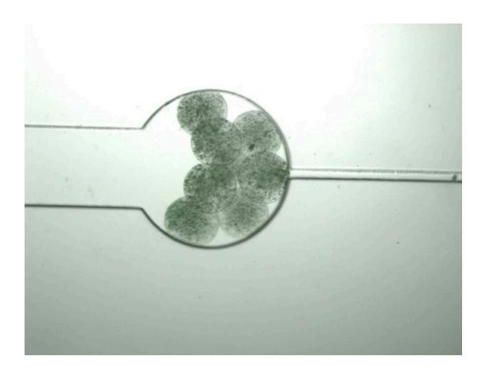
'Swarmbots,' living cells engineered to produce monomer molecules, grow until they sense their population density has reached a certain level, whereupon they burst open, allowing the monomers to mingle and self-assemble into a composite polymer. Credit: Zhuojun Dai
