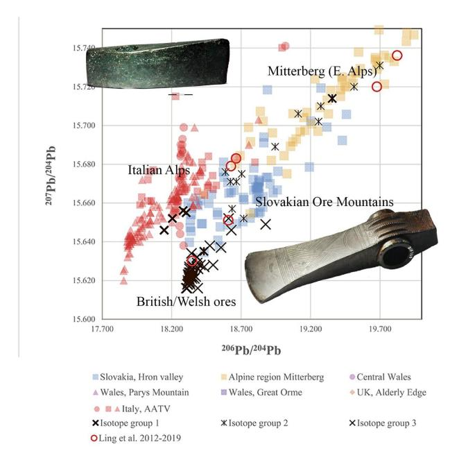
The lead isotope plot of the over 65 shafthole axes analyzed in this study dating to the end of the first Bronze Age period 1600 BC. This amount of data exceeds the previous analyses by ten times and for the first time allows to compare both axe types and understand their development. Credit: No credit
