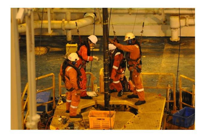
Drilling. Metal shafts extend the reach of the drill as it burrows below the seafloor. Credit: Kinoshita et al.
