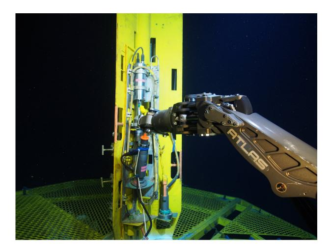
Drill inspection. A robot manipulator arm inspects the equipment underwater. Credit: Kinoshita et al.
