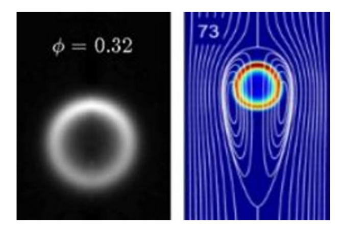
Left, cross-section of a flame ball in a mixture of hydrogen, methane and air at elevated pressure; right: Simulation of a flame ball residing inside a vortex. Credit: Eindhoven University of Technology
