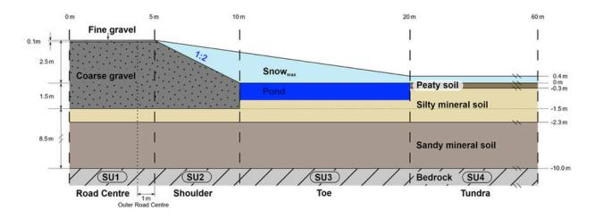
This diagram models half a road in cross-section from the road center to the adjacent tundra. The graphic illustrates the subdivision into four structural units (road center, shoulder, toe and tundra). The grayish area with black dots represents the road embankment. The light blue shading indicates potential maximum snow height. The dark blue area illustrates ponding next to the road. Credit: Image distributed under Creative Commons 4.0 International
