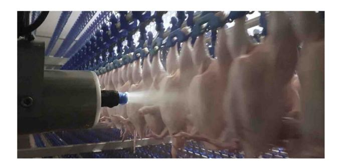
ChillBact's specialised nozzles, which they call ice guns, pump out a fine snow to cool hard-to-reach parts of a carcass. Credit: Thor Ice Chilling Solutions
