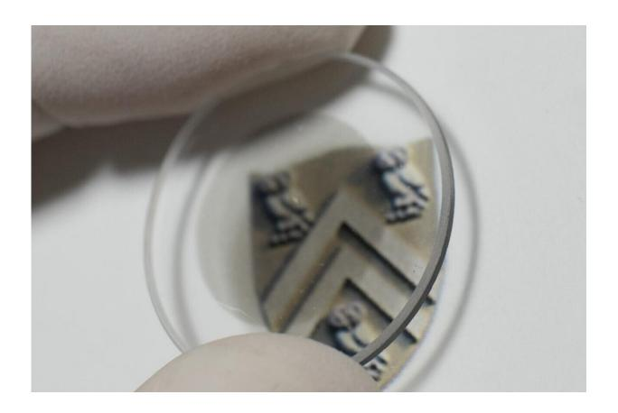
Ultrathin, broadband polarization rotators are made possible by ultrathin carbon nanotube films developed at Rice University in 2016. The films of highly aligned single-walled nanotubes were first made in 2016. Credit: Kono Laboratory/Rice University
