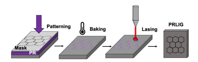
Rice University chemists have adapted their laser-induced graphene process to make conductive patterns from standard photoresist material for consumer electronics and other applications. Credit: Tour Group/Rice University
