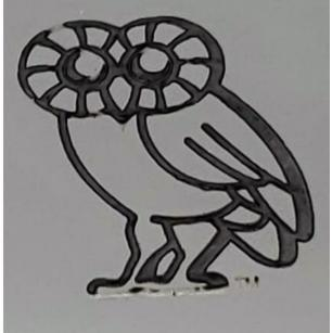
A laser-induced graphene Rice Owl is surrounded by photoresist material at left and stands alone at right after the excess photoresist is washed away with acetone. Rice University scientists are using the process to create micron-scale lines of conductive graphene that could be useful in consumer electronics. Credit: Tour Group/Rice University
