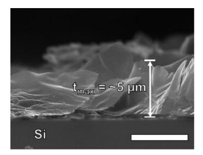
A scanning electron microscope image shows a cross-section of laser-induced graphene on silicon. The graphene was created at Rice University by lasing a photoresist polymer to make micron-scale lines that could be useful for electronics and other applications. The scale bar is 5 microns. Credit: Tour Group/Rice University
