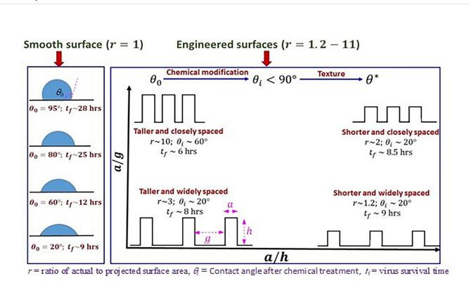
Surfaces with taller and closely packed pillars with a contact angle of around 60 degrees show the strongest antiviral effect or shortest drying time. Credit: S. Chatterjee, J.S. Murallidharan, A. Agrawal, and R. Bhardwaj
