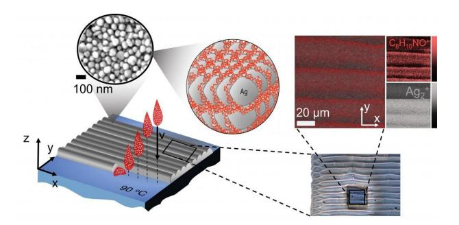
(left) Digital inkjet printing of inks containing metal nanoparticles with in-situ solvent evaporation (pinning). (right) Optical and chemical images of a printed layer of silver nanoparticles showing organic residues at the surface Credit: Gustavo Trindade
