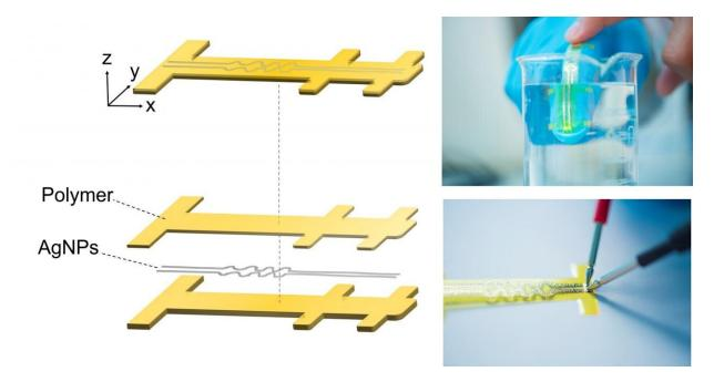
A multi-material inkjet 3D printed prototype of an encapsulated strain sensor used in the study Credit: Gustavo Trindade
