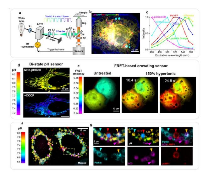
a, Schematic of the setup. Full-frame spectral micrographs are obtained by the synchronized fast modulation of the excitation wavelength in consecutive
