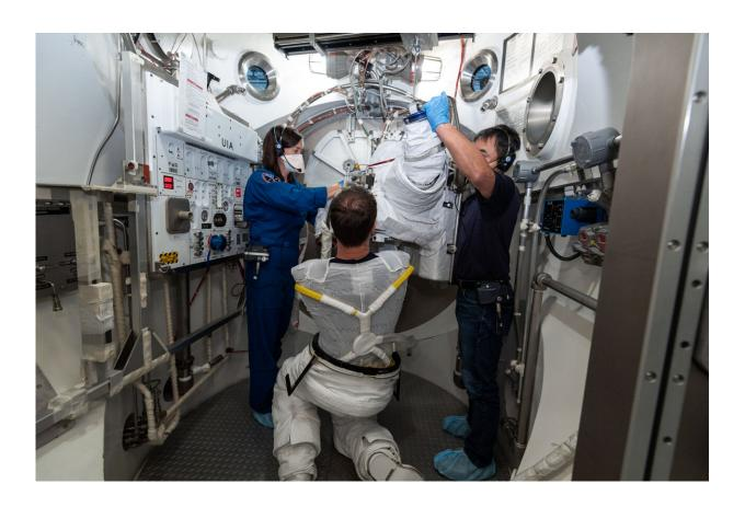
ESA astronaut Thomas Pesquet putting on his External Mobility Unit (EMU) spacesuit, with his Liquid Cooling and Ventilation Garment visible. Thomas donned the spacesuit fit check in the Space Station Airlock Test Article (SSATA) in the Crew Systems Laboratory at NASA's Johnson Space Center in September 2020, ahead of his Expedition 65 mission to the Intermational Space Station. Credit: NASA-Robert Markowitz
