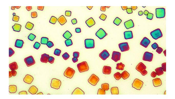
Optical microscopy image of large cubic superlattices. Such superlattices are potential candidates for use as highly energy-efficient,ultrafast light emitters. Credit: Empa
