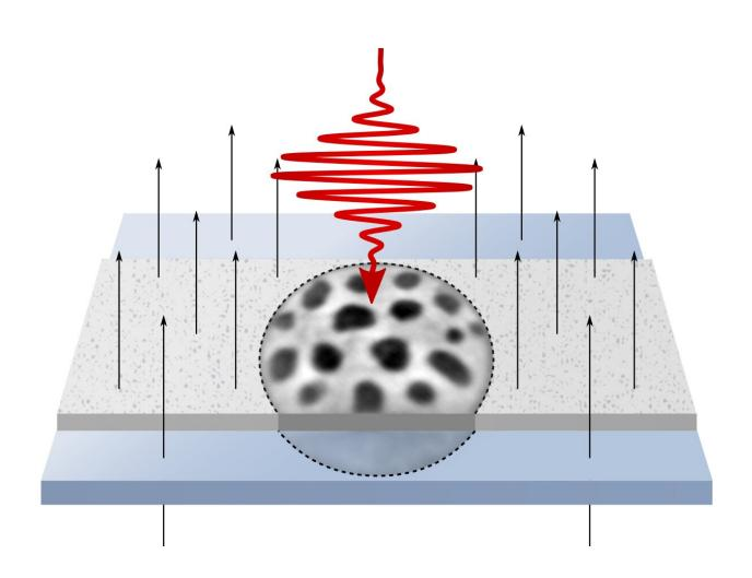
Fig. 1: A single laser pulse of appropriate intensity can create random skyrmion patterns with a density defined by an external magnetic field (thin arrows). This scheme of laser writing of skyrmions may be used as an ultrafast "skyrmion reshuffler" for stochastic computing. The area surrounded by the dashed line marks the field of view of the x-ray microscope used to see the magnetic skyrmions appearing as black dots. The field of view is 1  $\mu$ m in diameter. Credit:
