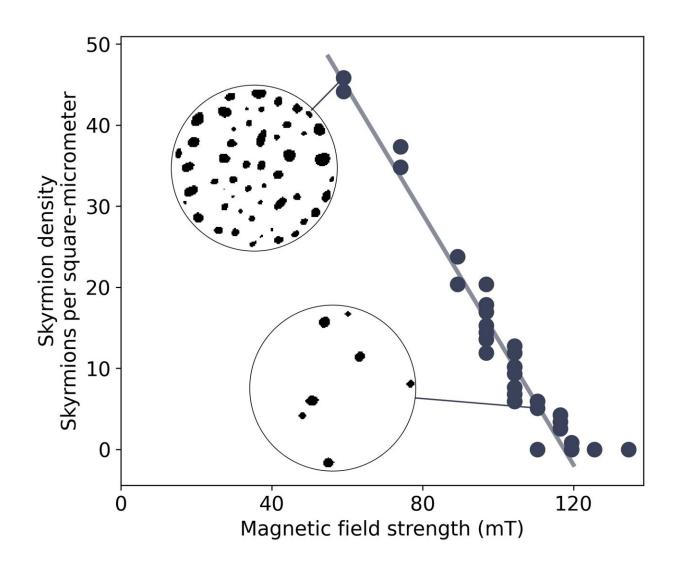
Fig 2: The density of skyrmions as a function of the external magnetic field. As the field decreases the skyrmion density increases in a linear manner. The inset images show examples of the skyrmion patterns created by the laser pulse, the field of view is  $1.5 \mu m$  in diameter. Credit: Forschungsverbund Berlin e.V. (FVB)
