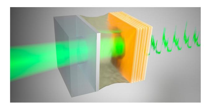
Two mirrors with a drop of oil in between form a non-linear optical cavity, in which stochastic resonance was observed. By modulating the position on one of the mirrors, the laser light (approaching from the left) is turned into a signal (right). An optimum amount of noise amplifies this signal when the conditions of stochastic resonance have been met. Credit: Henk-Jan Boluijt (AMOLF)
