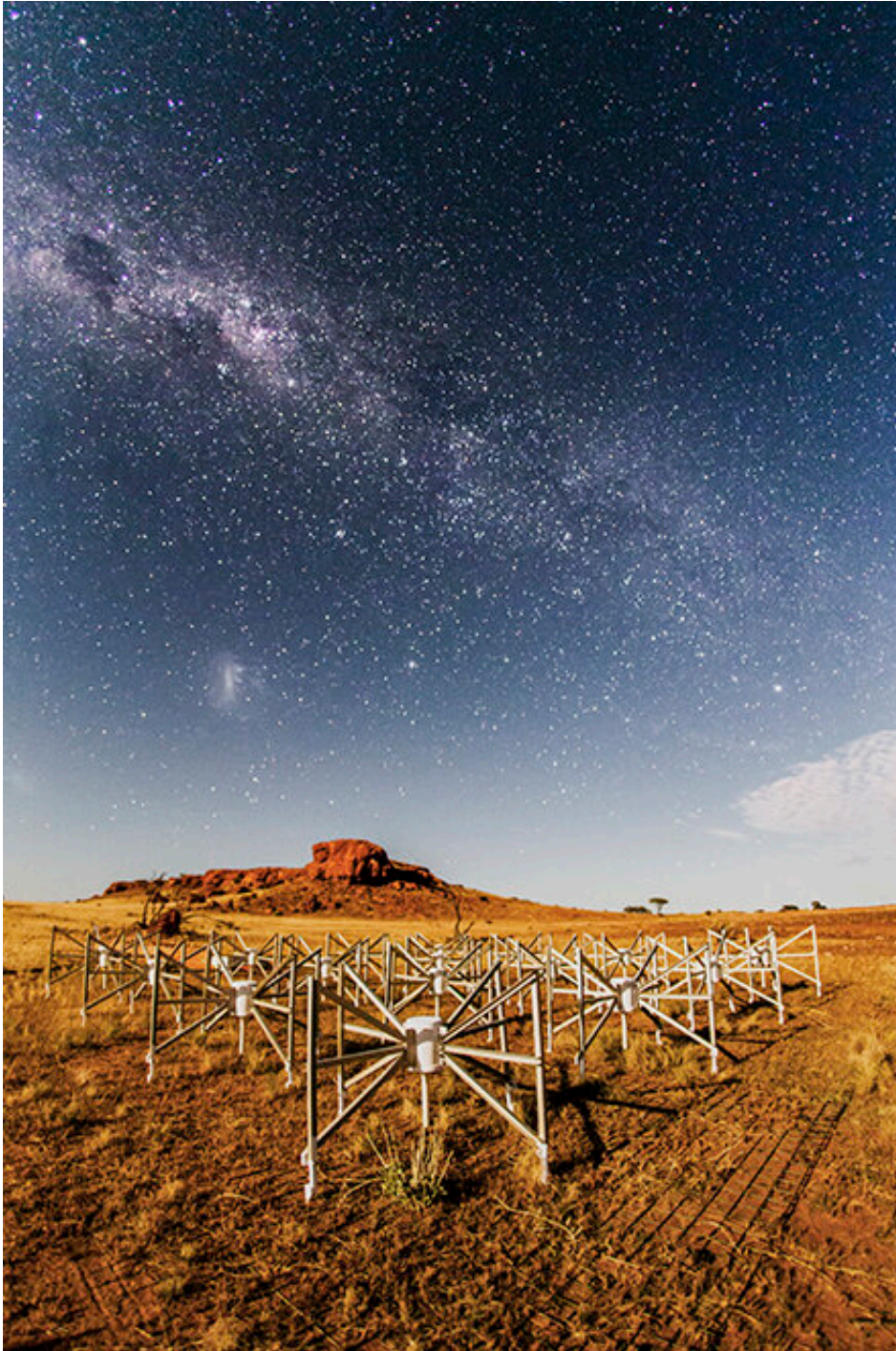
One of 256 tiles of the Murchison Widefield Array (MWA) radio telescope. Credit: Pete Wheeler, ICRAR
