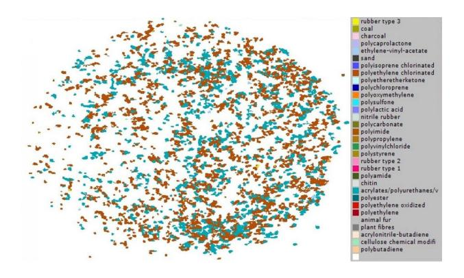
This image is generated by siMPle, an FTIR particle-analysis software, after comparison of the acquired particles spectra with a reference database. Credit: University of Portsmouth
