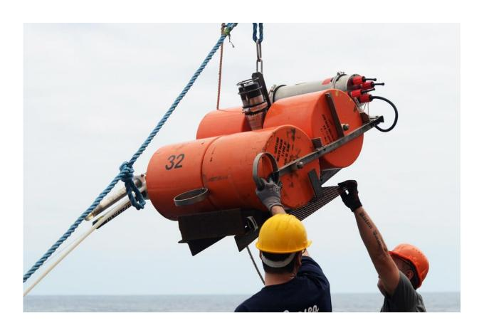
For a total of two years, 15 ocean bottom seismometers off northern Chile recorded aftershocks from the 2014 Iquique earthquake. Credit: Jan Steffen/GEOMAR
