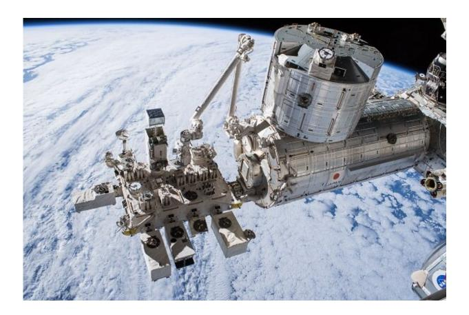
The suite of Earth-observing payloads attached to the Japanese Experiment Module is shown as the International Space Station orbits over the southern Pacific Ocean east of New Zealand. Credit: NASA
