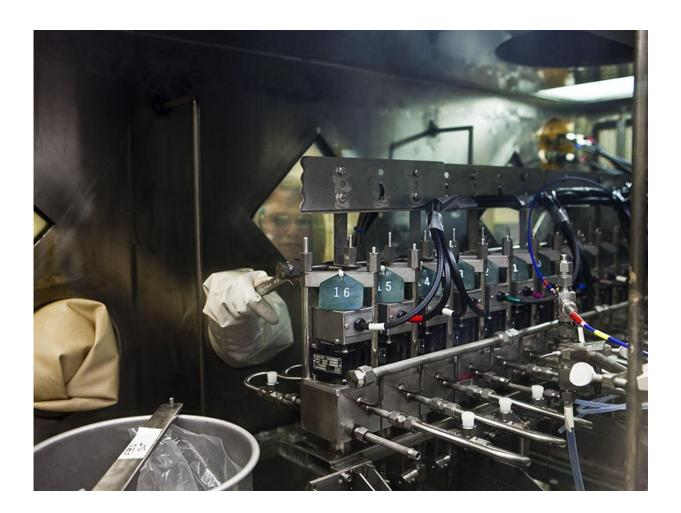
For recycling, spent nuclear fuel is fed into a chemical processing system that separates actinide elements that can be recycled as mixed-oxide fuel to produce more electrical power. At PNNL, this research is done in the Radiochemical Processing Laboratory, a Hazard Category II non-reactor nuclear research facility. Credit: Andrea Starr | Pacific Northwest National Laboratory
