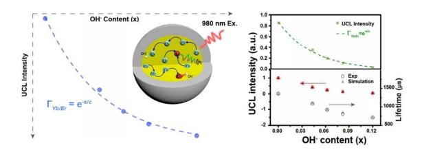
Experimentally observed exponential relationship between the dependence of upconversion luminescence intensity on internal OH- impurities. The image at bottom right represents a comparison between experiments and theoretical simulations. Credit: HIMS
