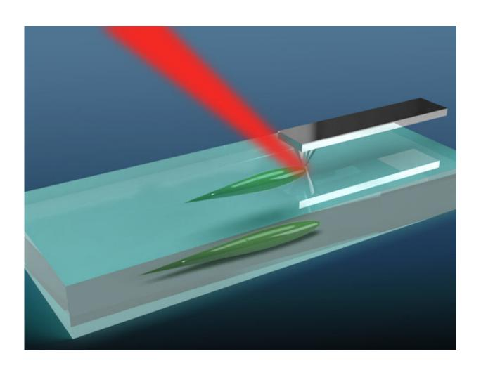
With hyperspectral near-field optical mapping, an infrared light beam can reveal nano-level imperfections and damage that weakens the glass sample. Credit: Elizabeth Flores-Gomez Murray, Penn State MRI
